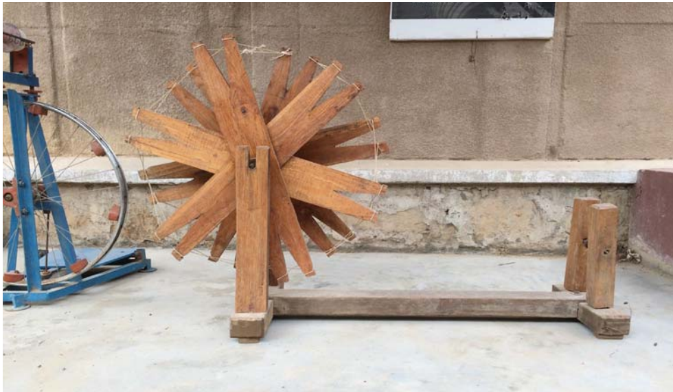
Figure 33: Kapur, H. (2016). Traditional Charka for khadi yarn spinning
