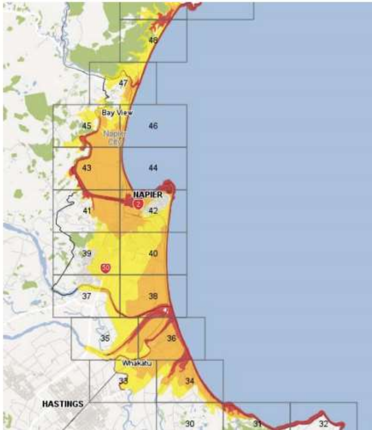
Figure 2. Overview of wider Napier Tsunami Evacuations Zones, showing the three zones of red - shore-exclusion zone; orange - area evacuated in distant and regional-source official warnings; and yellow – evacuation for all maximum credible tsunami (MCDem, 2008). (Source: Hawke’s Bay Regional Council and Hawkes Bay Civil Defence Emergency Management Group).
