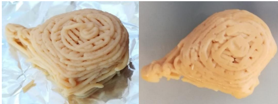
Figure 38. Printed 20C meat analogue with a drumstick shape at optimized parameters (1.54 mm nozzle, 10 mm/s & 100 % infill). Raw (left), cooked in boiling water for 10 min (right).
