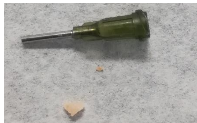
Figure 25. Big particles in chicken blocked the 1.54 mm nozzle during forward extrusion test.
