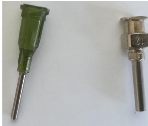
Figure 10. Two nozzles used for 3D printing in this study: 1.54 mm diameter (left) & 2.16 mm diameter (right).
