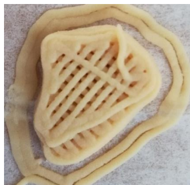
Figure 37. Printed 20C meat analogue with a nugget shape at optimized parameters (1.54 mm nozzle, 10 mm/s & 100 % infill).
