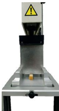
Figure 4. Slice shear force measurement using a flat blade.
