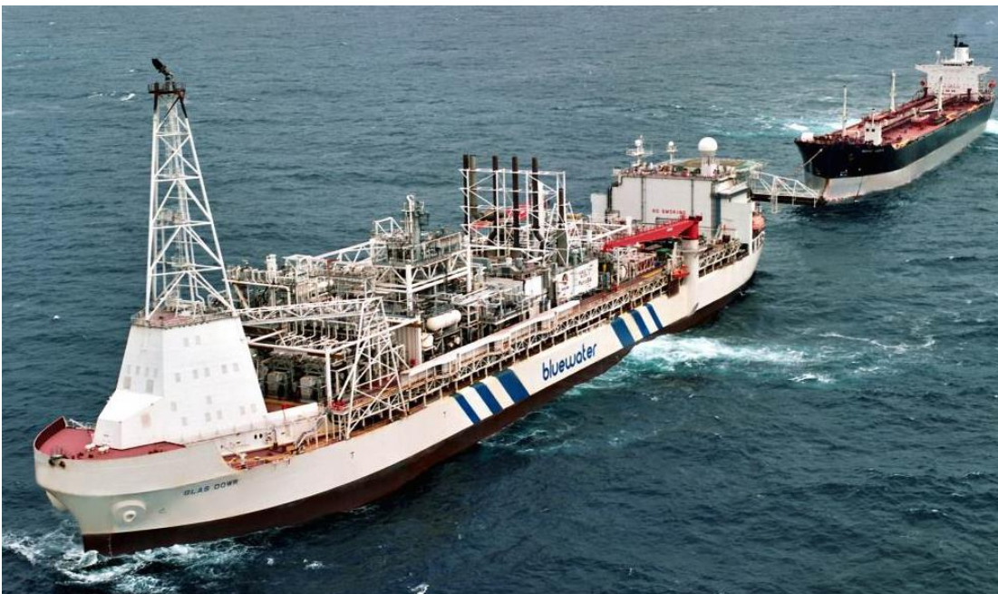
Figure 3: Blue Water Glas Dowl Floating Production Storage and Offloading (FPSO) vessel. Source: (La'o Hamutuk, 2016, p. 1).
