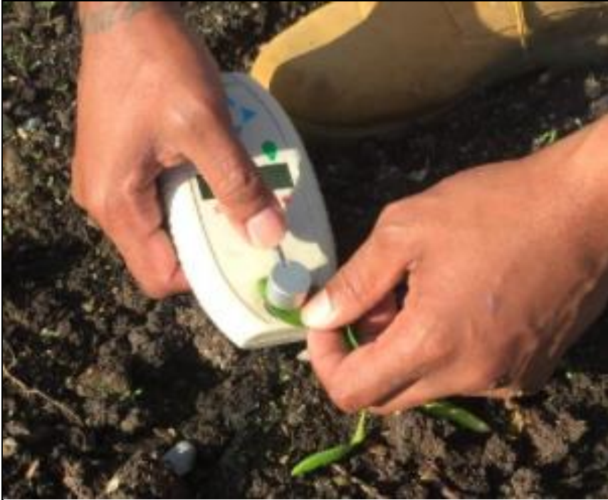
Figure 4. 7 Operation of the CCM-200 plus (chlorophyll content meter) on spinach. Joeli Savou, Palmerston North.
