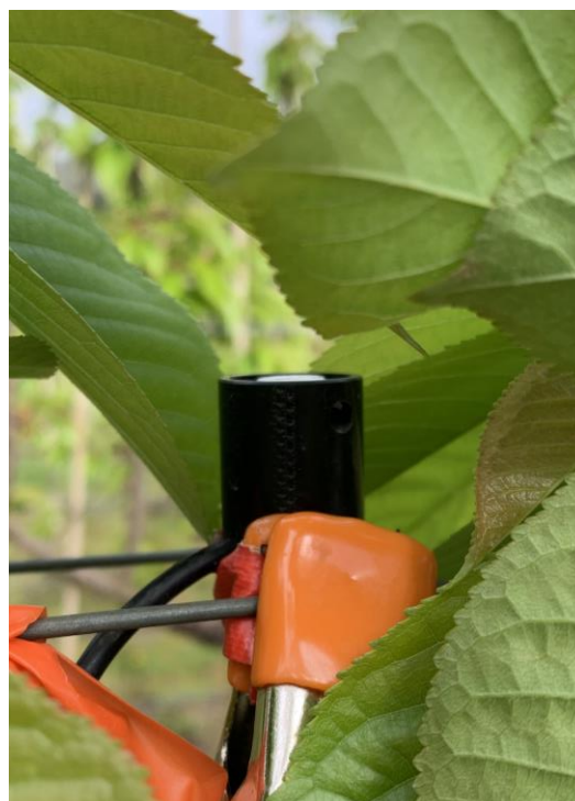
Figure 6: Photosynthetically active radiation (PAR) sensors developed in New Zealand by Tranzflo (Tranzflo, Palmerston North).
