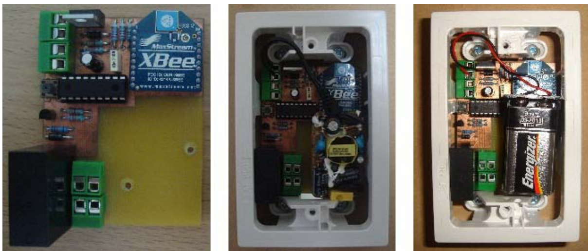
Figure 6.7: Various assemblies of the second switch
