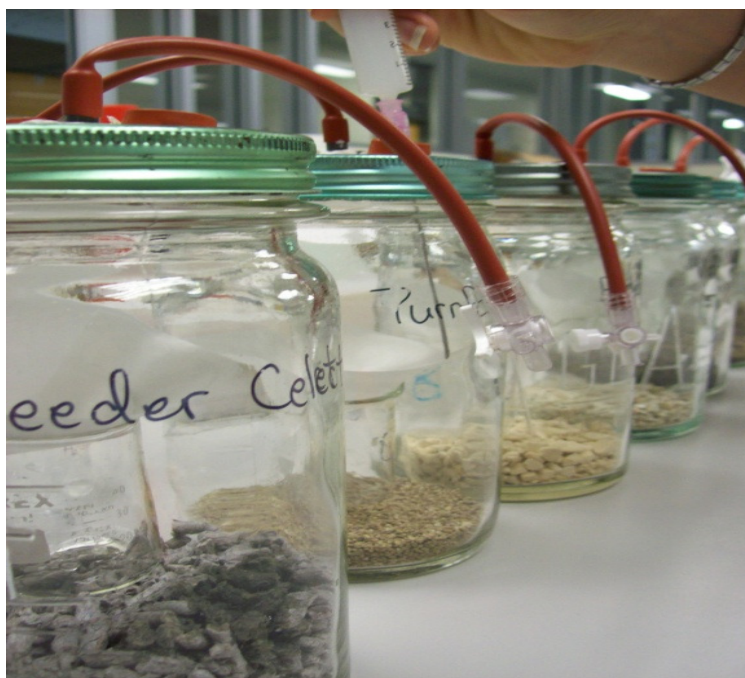
Figure 6.3: Experimental apparatus to show how ammonia was dispensed on to each cat litter.
