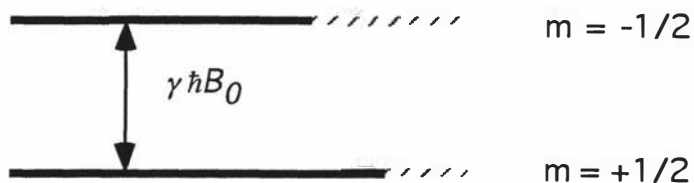
Figure 2.1: Schematic representation of the energy levels for an I = 1/2 spin in a magnetic field B_0 . The energy levels can be calculated from eqn (2.6) and the populations from eqn (2.20)
