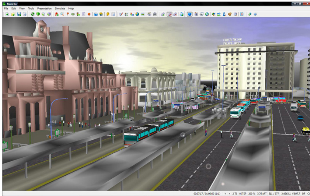
Figure 1: Paramics Modeller traffic simulation running, showing three dimensional representation using the available graphics libraries to preview buildings around the traffic network, as well as traffic members such as cars, trucks, public transport and pedestrians [13]
