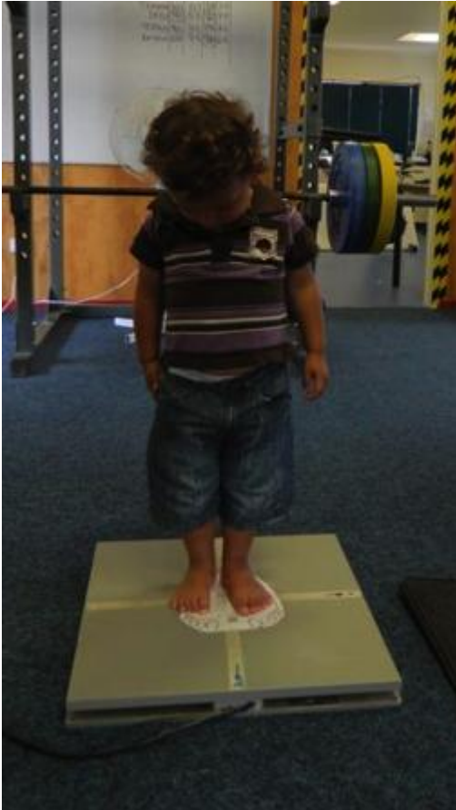
Figure 3.5. Photograph of child standing on force plate.
