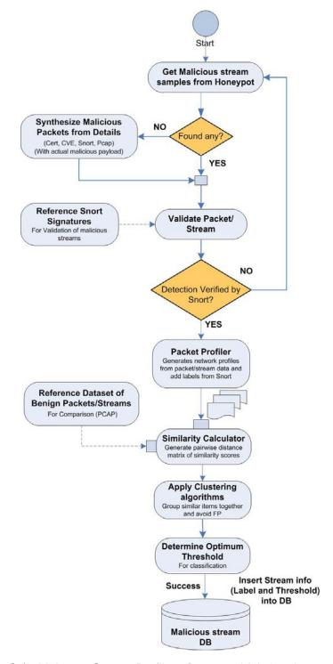
Figure 3.1: Malicious Stream Profiler: Create and label malicious streams
