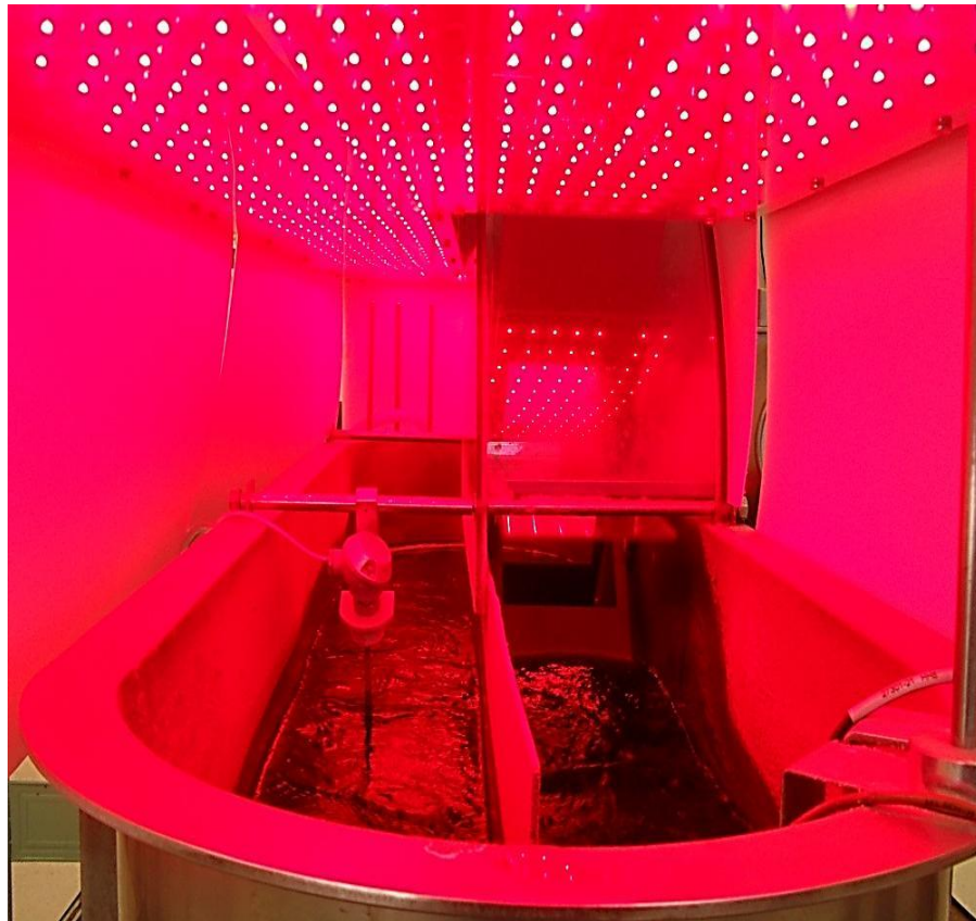
Figure 3.6 Raceway with LEDs in day mode of operation.
