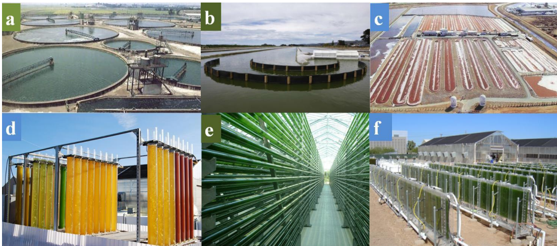
Figure 2.6 Some designs of open and closed microalgal production systems: a) Centre-pivot ponds used for the production of Chlorella , Taiwan ( www.pureplanet.de ); b) Algae wastewater treatment raceway pond at the NIWA's research site, Christchurch, New Zealand (National Institute of Water and Atmospheric Research Ltd); c) Dunaliella bardawil cultivation in raceway ponds (Nature Beta Technologies Ltd, Eilat, Israel, subsidiary of Nikken Sohonsa Co. Gifu, Japan); d) Bubble column photobioreactors growing algal strains for different pigments at Arizona State University's Polytechnic campus in Mesa, Arizona, USA; e) Tubular photobioreactor used for biomass production in Klötze, Saxony Anhalt, Germany (© Bioprodukte Prof. Steinberg GmbH); f) Plate-type photobioreactors, NanoVoltaicsk Inc. ( www.nanovoltaiics.com ), Arizona, USA.
