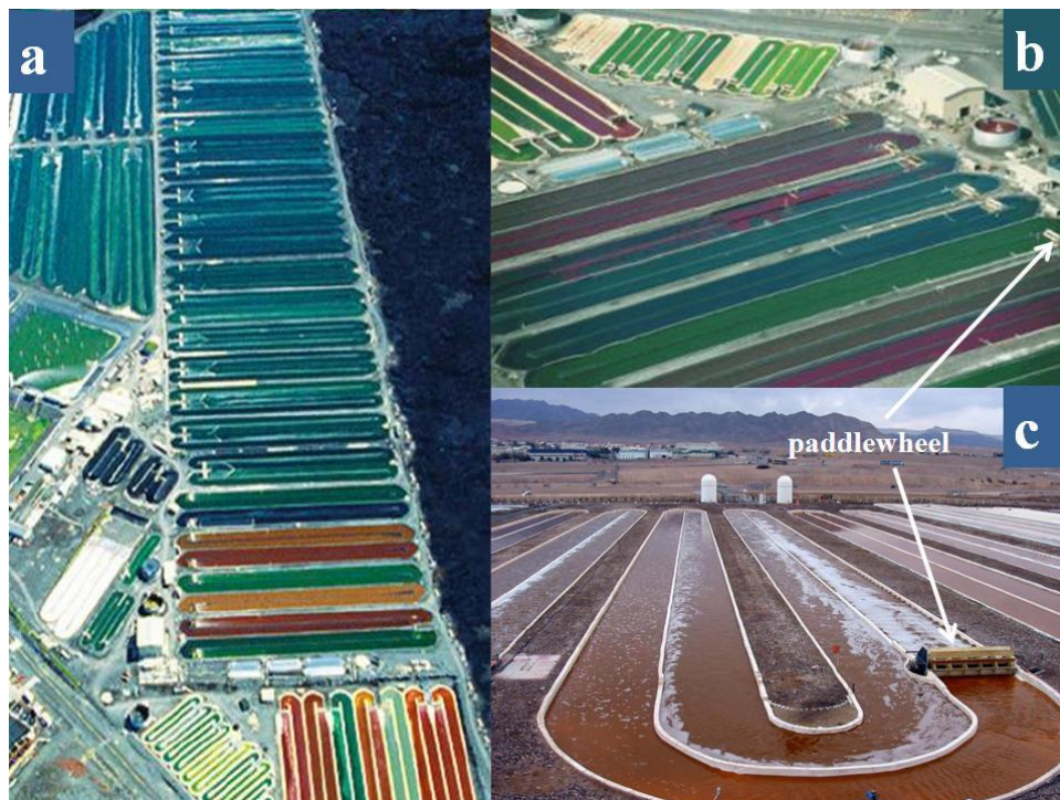
Figure 2.7 Commercial algal biomass production in raceways: a) and b) Cultivation of Spirulina (a blue-green cyanobacterium) and Haematococcus pluvialis (an orange pigment producing green alga) by Cyanotech Corporation, Kona, Hawaii ( www.cyanotech.com ); c) Dunaliella bardawil cultivation in raceway ponds (Nature Beta Technologies Ltd, Eilat, Israel, subsidiary of Nikken Sohonsa Co. Gifu, Japan).
