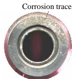
Figure 5-7. Corrosion trace on membrane adapter
