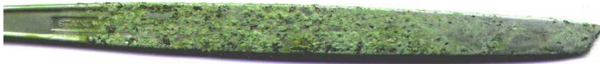
Figure 5-9. Corrosion of the stainless steel anode after electrolyzing the Alamin solution for 24 hours. Alamin particle concentration was 0.7%(w/v). The electrode current was 0.08A (equivalent to 80\text{A/m}^2 ). Voltage applied was 10V (equivalent to 36\text{V/cm} of electric field strength).
