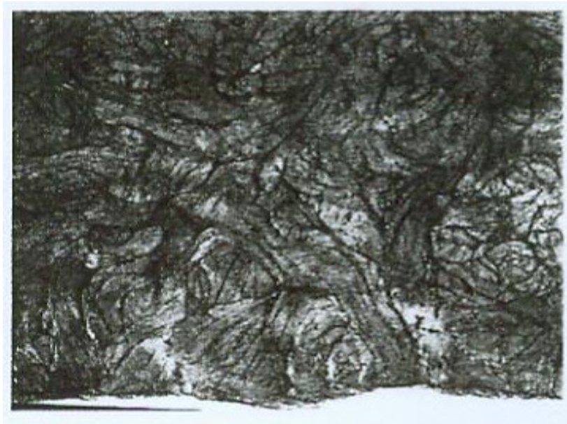
Figure 1.4.2: Cross Section of tight leather with less space between the fibres (LASRA)
